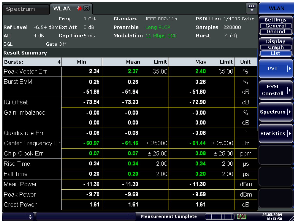
Fig. 3-13: Result summary list for measurements on DSSS/CCK/PBCC signals
