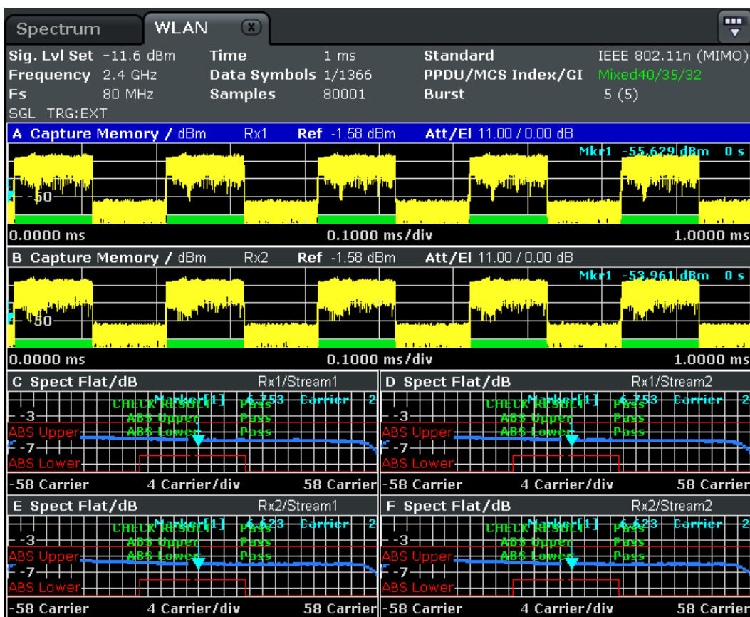
Fig. 4-2: Spectrum flatness result for IEEE 802.11n (MIMO) with 2 streams
